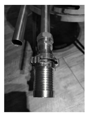
Step 4: Connect the Intex pump including the hoses to the coil (hoses and pump are not included).
